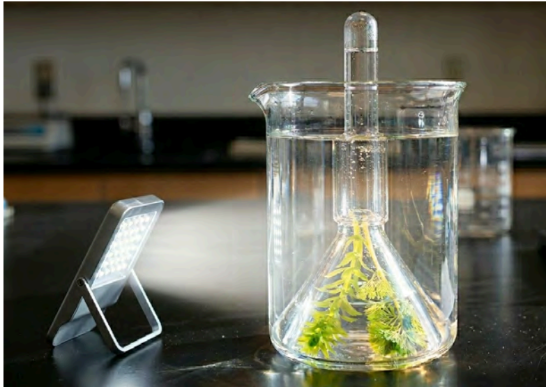
Figure 2. Experimental setting for measuring rate of photosynthesis. The experiment has been running for a while and oxygen has gathered in the test tube.
